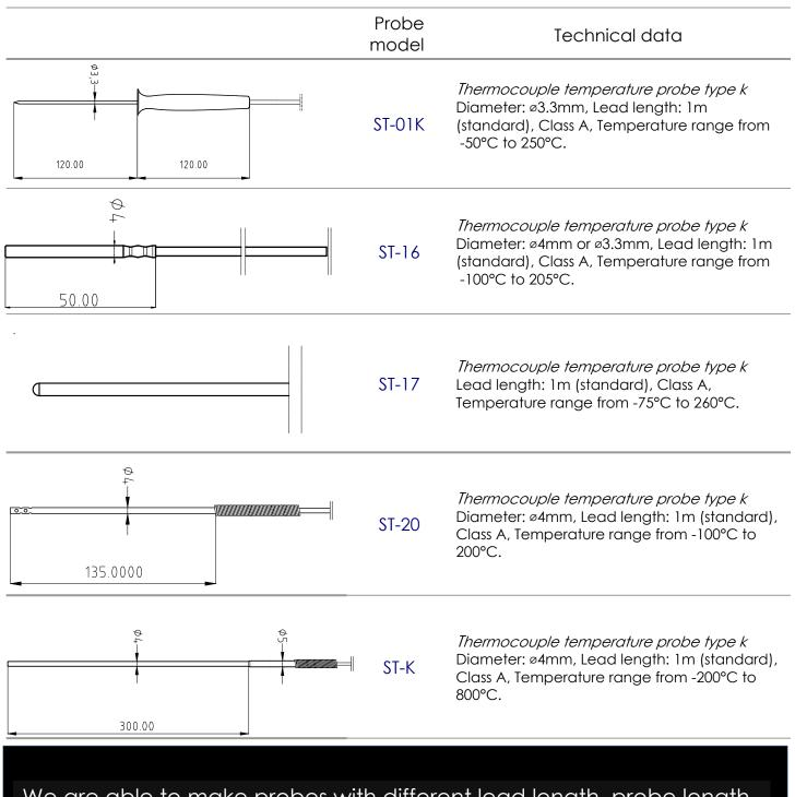
We are able to make probes with different lead length, probe length, probe diameter and sensors like PT100/PT500 depending on your needs.
